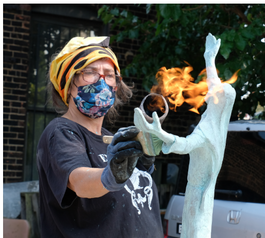
Lisa Kenion, Sr. Megan's foundry colleague, heats the metal as the chemicals are applied to the sculpture.
